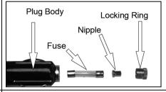
Replace the 15A glass fuse and reassemble the plug.
